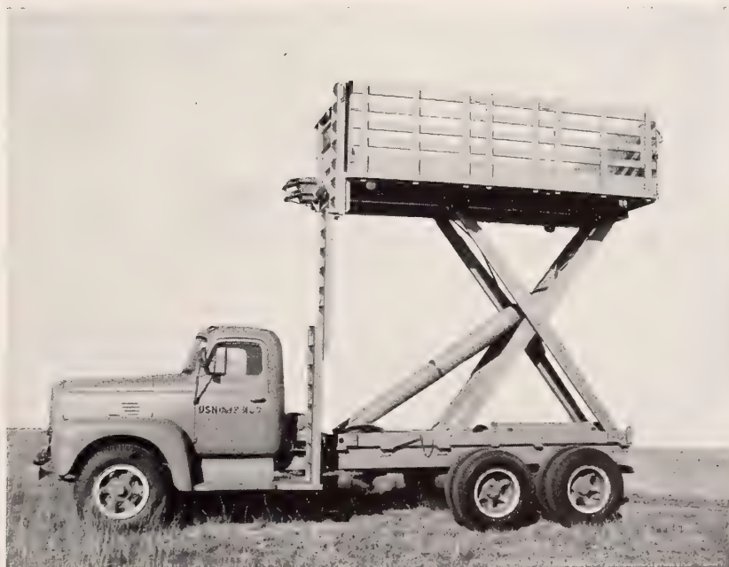
New type Cresci Extra Heavy Duty Hi-lift Cargo Loader now being produced for the U. S. Navy.
