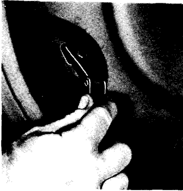
LINING CLEARANCE CHECK
